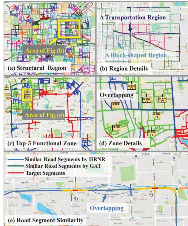
**Figure 4: Visualization of the learned representations for road segments, structural regions and functional zones. The colored lines denote road segments in the road network. Road segments with the same color correspond to one structural region or one functional zone.**
